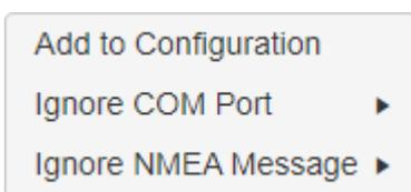
If you wish to add the discovered message definition to your current Working Configuration in **CFE** click *Add to Configuration*. The entire message and all it's **Data Fields** will automatically be added and broken out for you. Review it and don't forget to **Save** and **publish** for it to become active inside **ACQ**!
